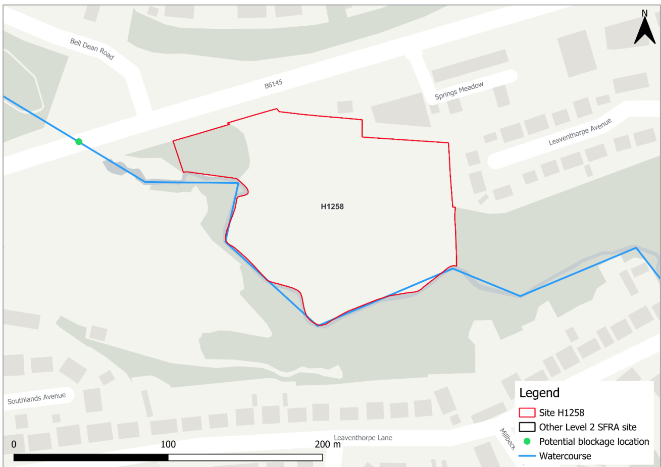
Figure 5-1: Potential blockage location
